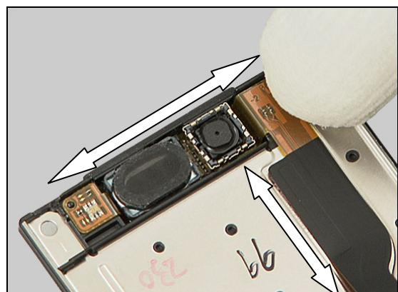
Insert the BtB end of the Slider Flex Module through the slot of the Slider Unit,
