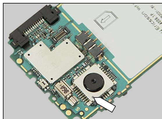
Insert the dentist hook into the corners of the Lid to release it,
