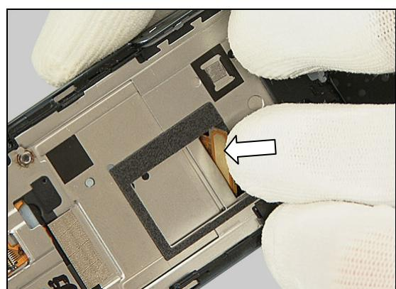
Use the Front Opening Tool to release the Slider Flex Module from the Sliding Unit.
