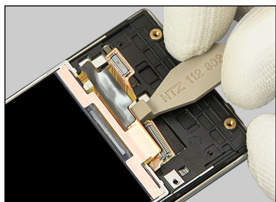
Remove the Display by lifting straight up.
