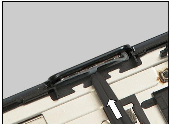
until the Volume Key is properly installed as shown from the inside,
