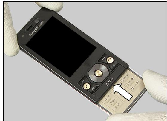
Push the knob lock in the direction of the arrow to unlock the Battery Cover.
