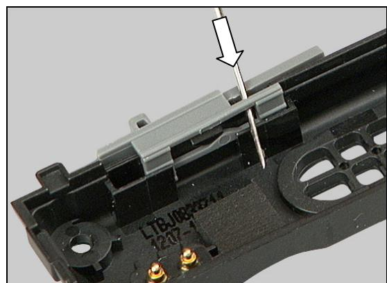
Pull upwards to release and remove the Knob Lock.
