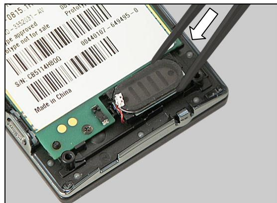
Press down with the flat end of the tweezers to make it securely attached.
