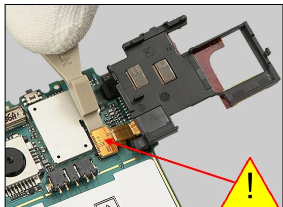
Remove the SIM Flex/Carrier Unit.
