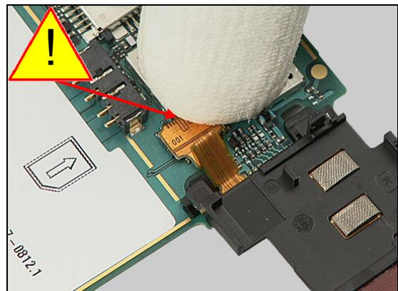
Turn the SIM Flex/Carrier Unit over the Main PBA.
