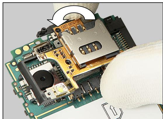
Press on both sides of the SIM Flex/Carrier Unit,
