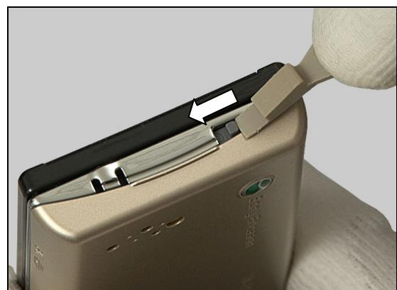
Insert the Plectrum to release the Battery Cover.
