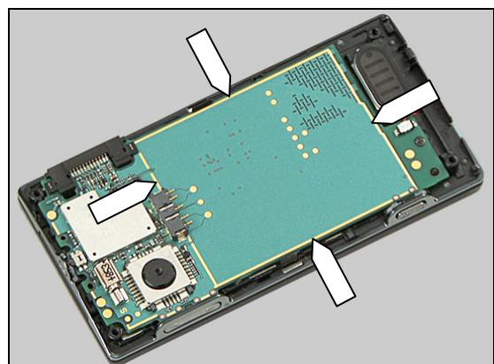
Place the new Core Unit Label inside the 'golden' frame as shown in the adjacent picture.
