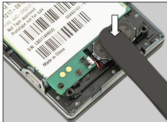
Connect the Loudspeaker by pressing its connector from the top into the Main PBA connector.
