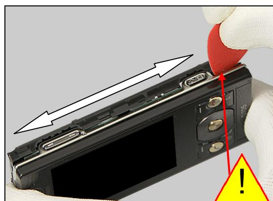
Remove the Rear Cover by lifting straight up.
