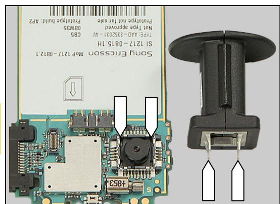
Insert the tool all the way into the camera socket with the Camera Removal Tool in the position shown in the picture.
