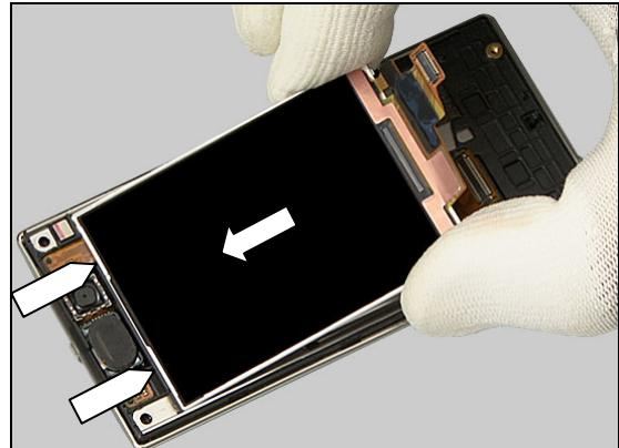
Push the Display down into its proper position.
