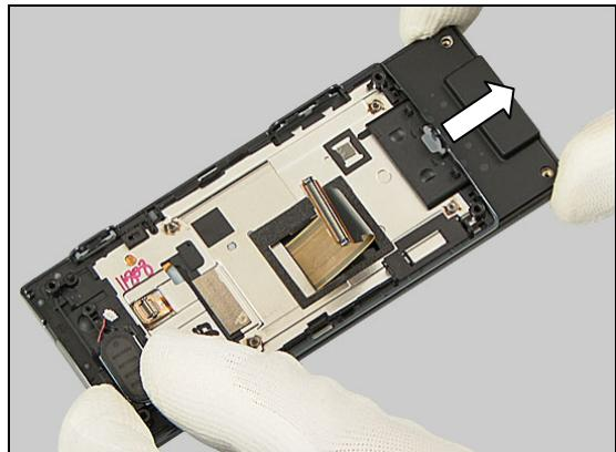
Apply 10 Ncm torque when tightening the two 1.6 mm black screws with the JCIS bit.
