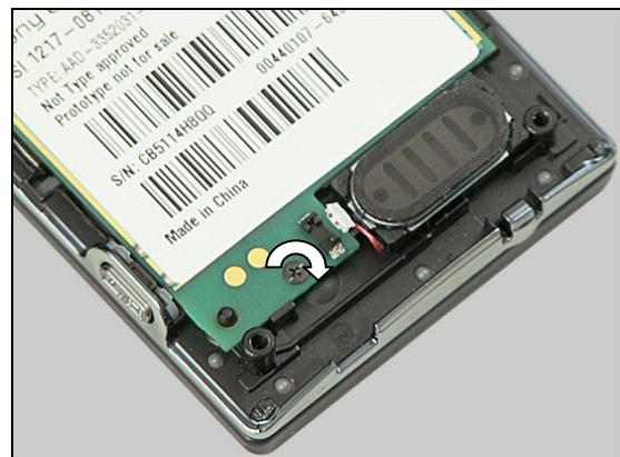
Connect the Loudspeaker by pressing its connector from the top into the connector of the Main PBA.
