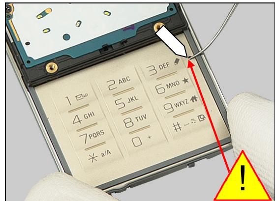
Gently peel the Keyboard off the Key Flex Module by using the tweezers.
