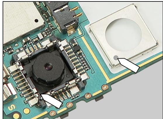
Place the Lid on top and in level with the camera,
