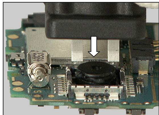
Wag the tool, as indicated by the double arrow, to release the Camera from its socket,
