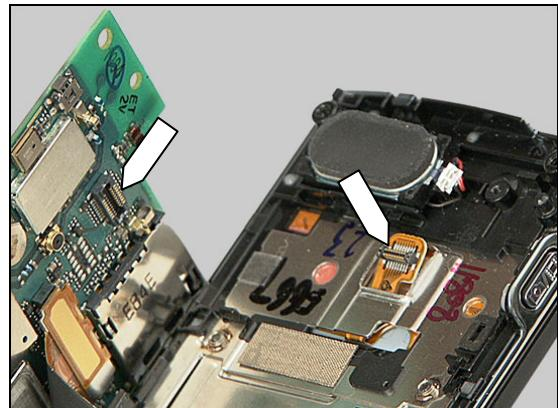
Hold the Main PBA in a slight angle and insert it at the top as indicated by the pointers and the arrow.
