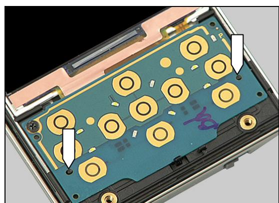
Attach the Dome Sheet and verify that the two holes are properly aligned with the pegs as described above and that the eight LEDs can emit light through the holes of the Dome Sheet (as indicated by the blue circles).
