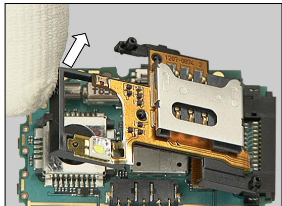
and use the Front Opening Tool to disconnect the BtB connector.
