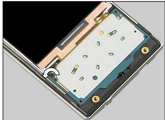
Insert the Plectrum as shown in picture to release the Navigation Key Unit,
