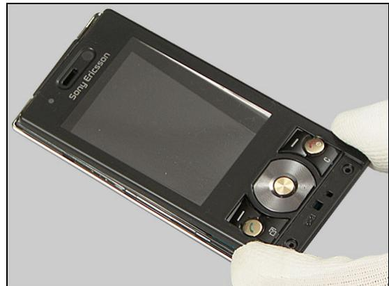
Press like this to snap this side of the Front Cover to the Slider Unit.
