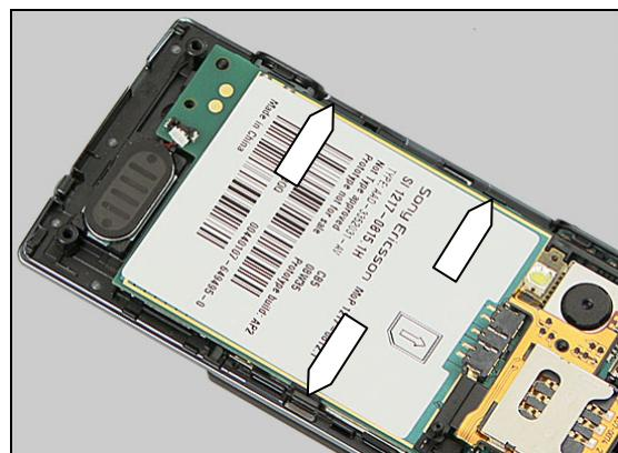
Release the Main PBA from the three hooks by using the Front Opening Tool.
