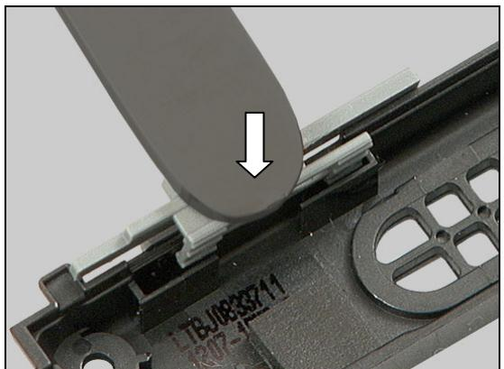
Check that the Knob Lock is properly installed by sliding back and forth.
