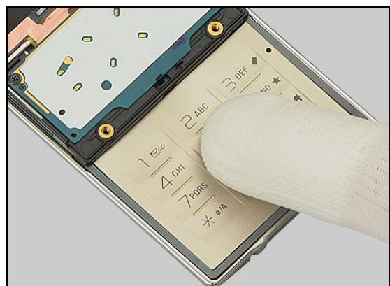
to make it securely attached to the Key Flex Module.
