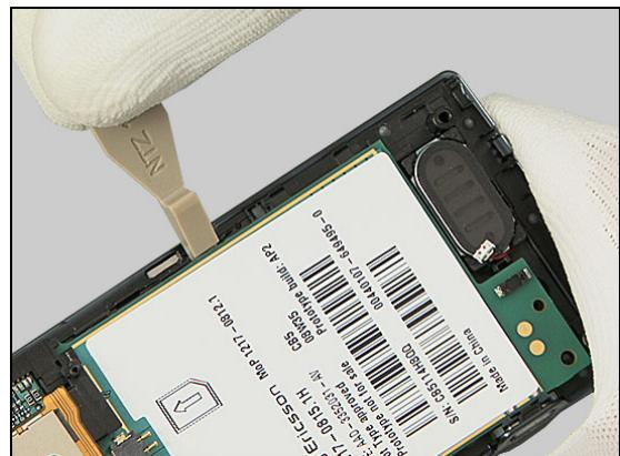
Raise the bottom of the Main PBA approximately 30° at the bottom,
