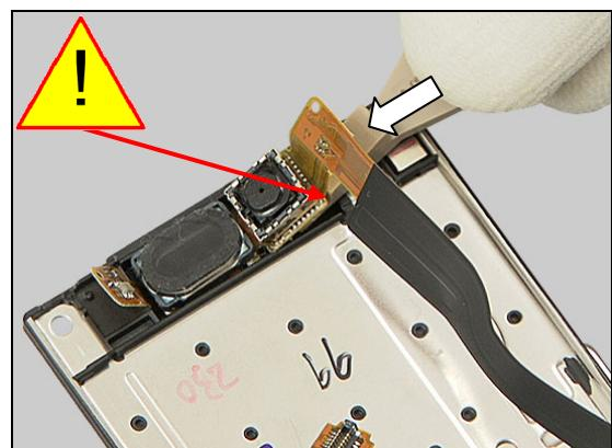
until the Slider Flex Module is entirely released and can be removed.
