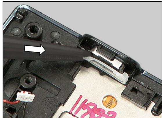
inside its corresponding pockets, and push by using the tweezers,
