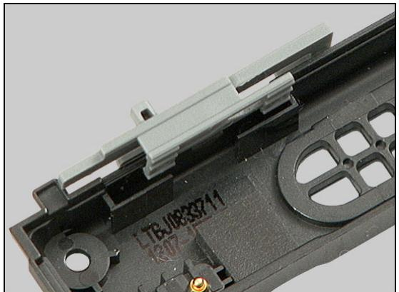
Press down with the flat end of the tweezers until it snaps into its proper position.
