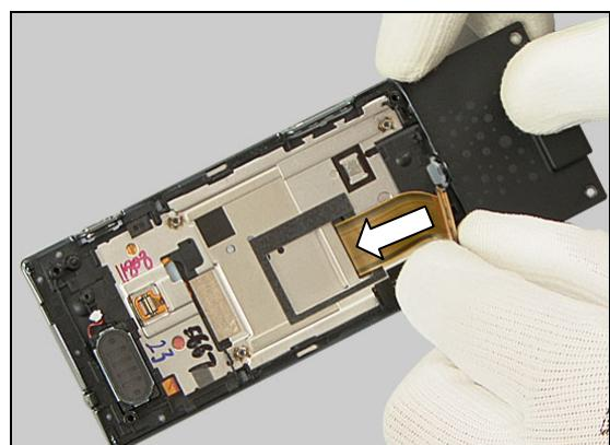
Turn the BtB connector in a slight angle to be able to make it pass through the slot.
