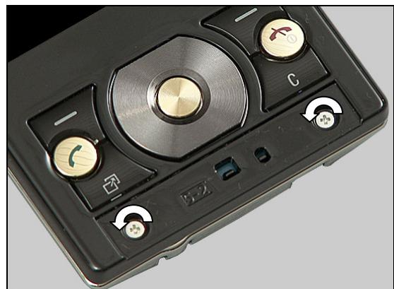
Insert the Plectrum as shown in picture and gently slide back and forth to release this side of the Front Cover.
