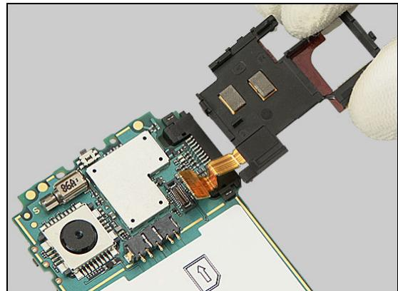
and connect its BtB connector to the Main PBA by using your finger.
