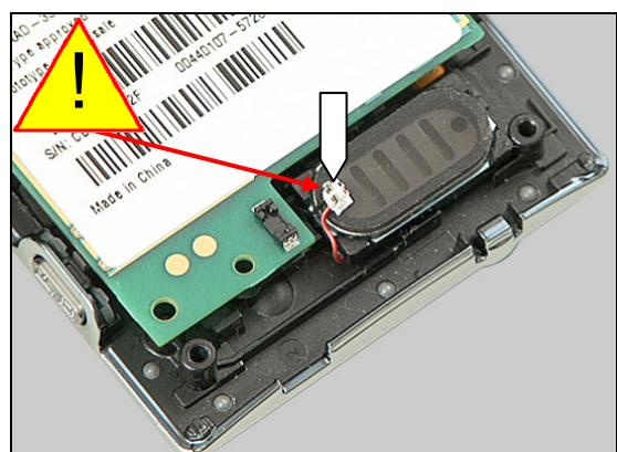
Press on both sides of the PBA to secure it to the Slider Unit.
