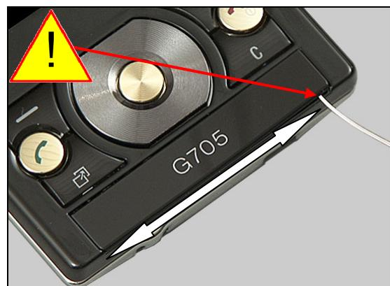
Carefully insert the needle type dentist hook underneath the Co-Branding and slide the dentist hook back and forth,
