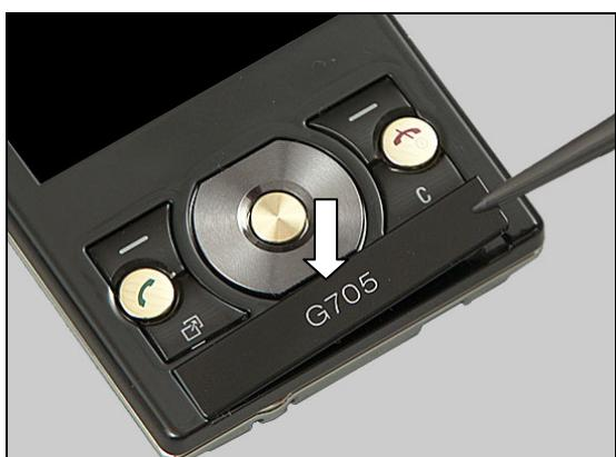
Press along the surface to make the Co-Branding securely attached.
