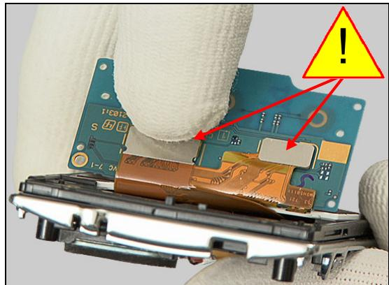
Turn the Navigation Key Unit back to its horizontal position.
