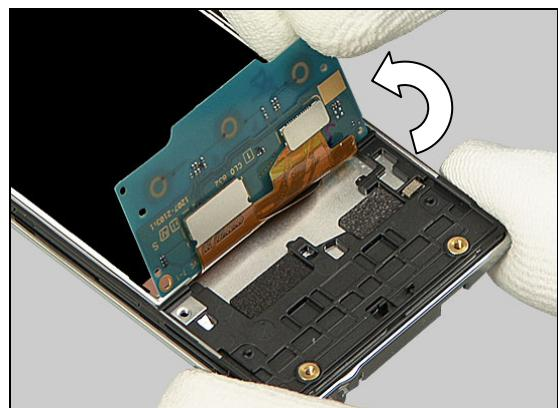
Use the Front Opening Tool to disconnect one of the two BtB connectors.
