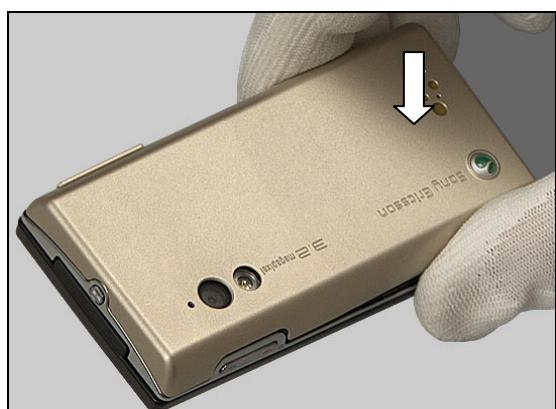
Press on both sides to make it snap onto the Rear Cover.
