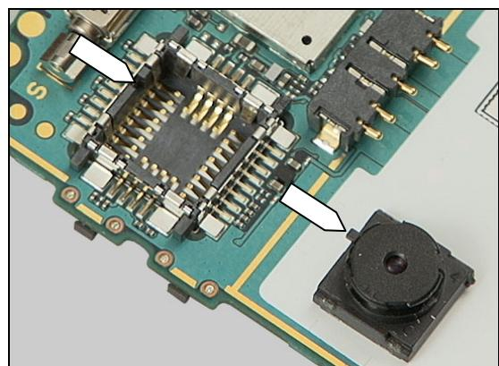
Place the camera inside and in level with the socket,
