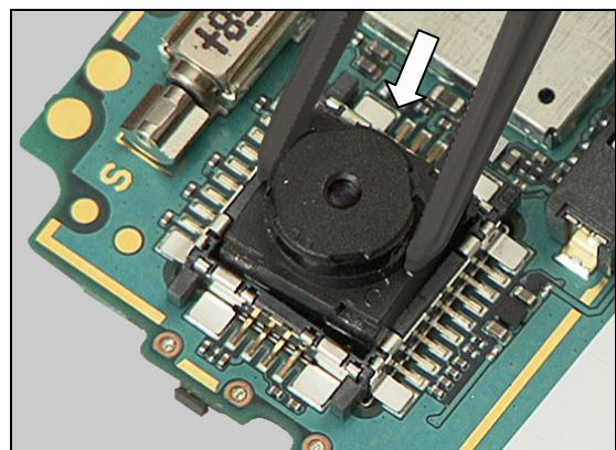
and press with your fingers, without touching the camera lens, to the bottom of the socket.
