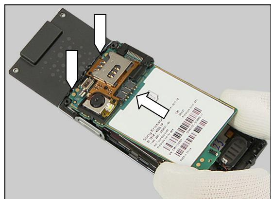
Before securing the Main PBA to the Slider Unit, check and, if necessary, move the Loudspeaker connector/cables to avoid that they become squeezed by the Main PBA.
