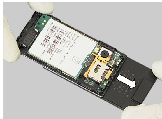
There are three snap hooks securing the Main PBA.
