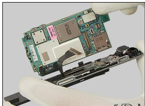
and connect the BtB connector by using your finger.
