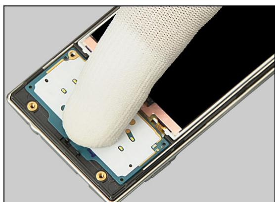
Apply 10 Ncm torque when tightening the 1.6 mm black screw with the JCIS bit.
