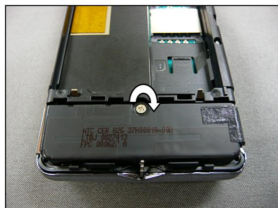
Use  $10.1 \pm 0.5$  Ncm ( $1.03 \pm 0.05$  kgf-cm) torque to tighten one screw with Philips screw driver.
