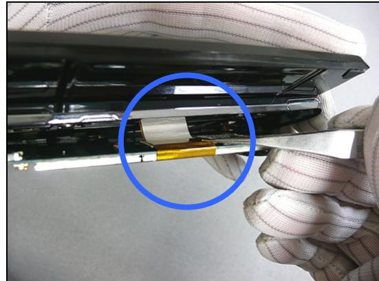
Use front opening tool to disconnect Rigid-Flex PCB.
