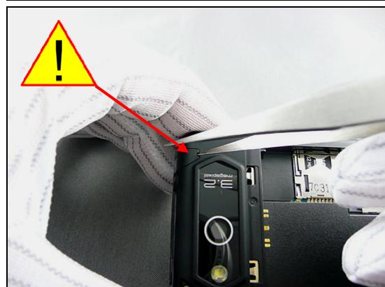
Use Torx bit no 6 to remove two screws.
