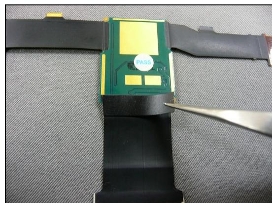
Stick one mylar on the rigid-flex PCB.
