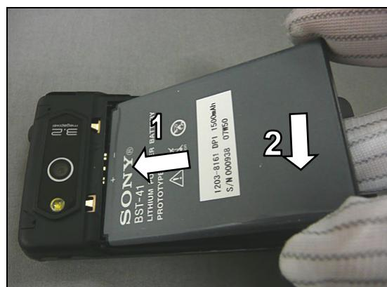
Follow the sequence shown in photo. Insert the battery cover and push it toward the top of the phone and then press the battery.
