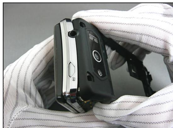
And then snap the rear bottom housing and keypad cover at USB connector side as shown in photo.
