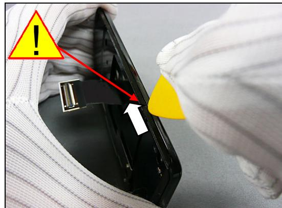
Insert the guitar pick as shown in picture and slide it along the arrow direction to unlatch the one snap hook. If necessary, slide back and forth until the snap hook is unlatched.
