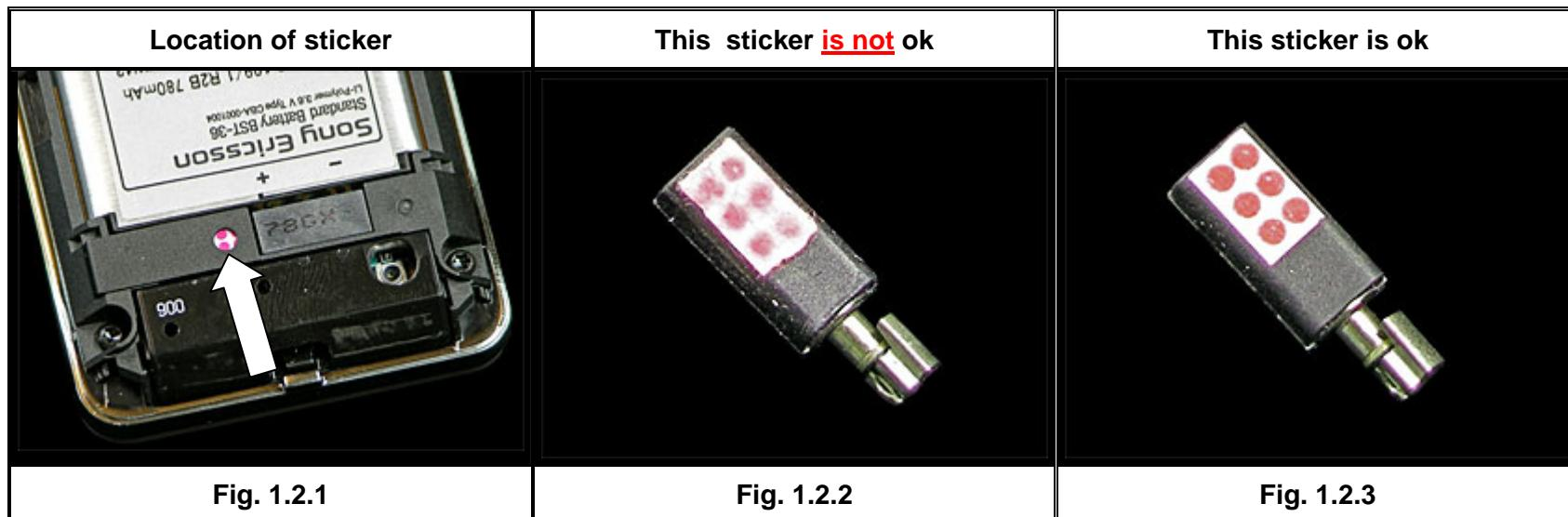
If the white indicator has been in contact with liquid, it turns into a blurred indicator. In this case you should check the phone for liquid damage (see point 1.2.1).
