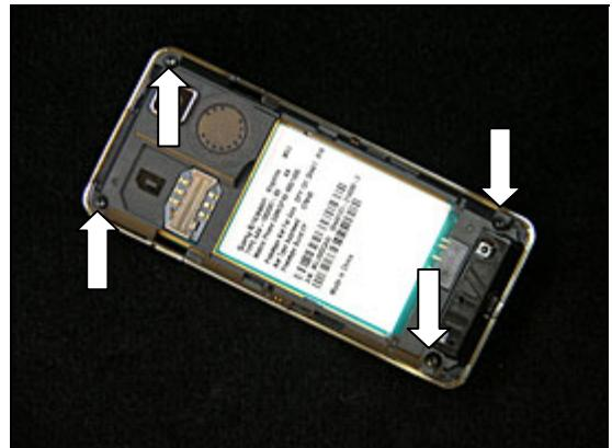
Use a guitar pick and slide along the side to release the snap hooks.
